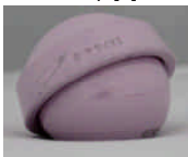
Figure 1: The alumina matrix composite hip replacement (AMC, commercially known as BIOLOX® Delta).
