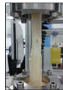
Figure 1. Specimens were potted in PMMA cement using bespoke fixtures and subjected to uniaxial failure testing.
