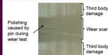
Figure 4: Surface of PEEK Optima® plates following damage simulation and 1MC wear simulation
