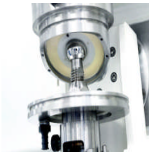
Fig. 2 Single station of the ProSim hip simulator (Simulator Solutions, UK) showing the mounted femoral head and the PE acetabular cup
