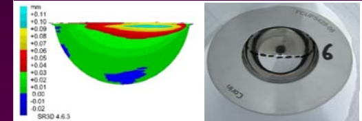
Figure 6: 3D reconstruction showing the shape, orientation and depth of the wear scar on the acetabular cup, positive values indicate wear.
