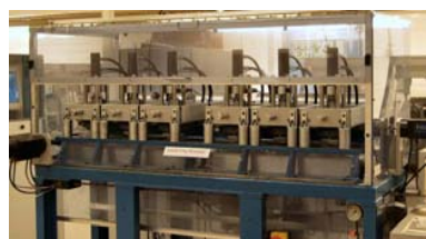
Figure 2: Leeds II Physiological Anatomical Hip Joint Simulator [6].
