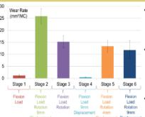
The measured polyethylene wear rate depended on the gait inputs applied to through the simulator
