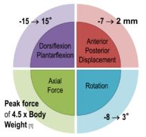
A gait profile was defined. Five combinations of inputs were tested for 2 million cycles (MC) with Stage 2 inputs repeated. Wear was quantified gravimetrically every MC.
