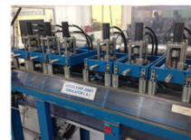
Six-station Leeds Mark II Physiological Anatomical Hip Joint simulator
