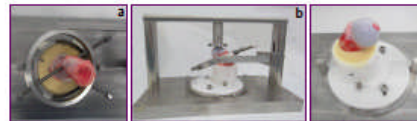
Figure 3: Femoral head potting: (a) aligning head with potted acetabulum; (b) positioning femur in test pot at correct centre height using jig; (c) femur potted in PMMA bone cement.
