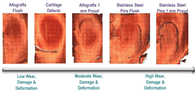
Figure 6: Schematic highlighting damage & wear observed in the experimental groups. Images are of the medial meniscus taken using an Alicona Infinite Focus optical profiler. Mean negative control group volume 0.089 mm 3 .
