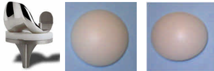
Figure 1: Components for the wear test (Left to right: Femur CR Sigma, round and oval dome patella buttons).
