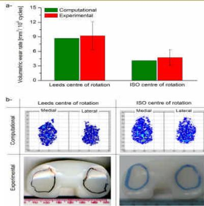
Figure 3: PFC Sigma fixed bearing computational and experimental (mean  $\pm$  95% confidence interval) wear rates [mm<sup>3</sup>/million cycles] (a), and wear scars (b).
