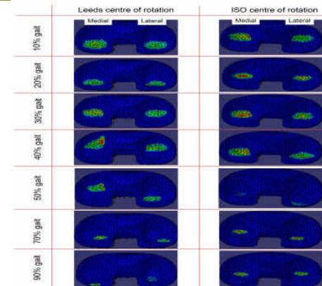
Figure 4: PFC Sigma fixed computationally predicted contact stress [MPa] (contact area [mm<sup>2</sup>]) at different % gait cycle, for Leeds and ISO CORs.
