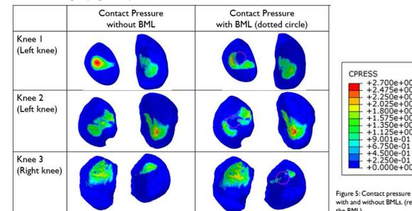
Figure 5: Contact pressure (MPa) maps for knee models with and without BMLs. (red circles indicate location of the BML).
