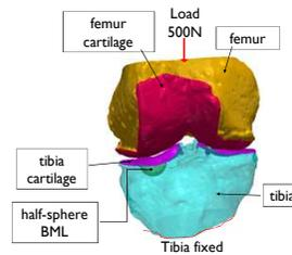
Figure 3: Schematic of finite element model set up showing bones, cartilage, load and boundary conditions.
