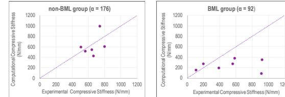
Figure 4: Graphs showing computational compressive stiffness plotted against experimental compressive stiffness for non-BML and BML groups.
