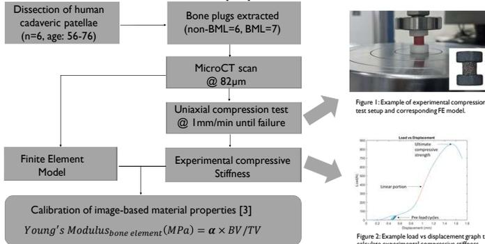
Figure 1: Example of experimental compression test setup and corresponding FE model.
