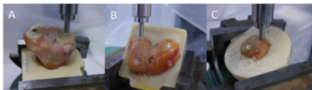
Figure 1: Samples mounted to Instron 3365 and push-in test being performed on (A) Medial and Lateral Tibial Plateau, (B) femoral condyles and trochlear groove, (C) Medial and Lateral patella
